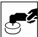
Dust and minor damage can be polished out after stated dry times. If baking, allow cool down of the object to ambient temperature.
