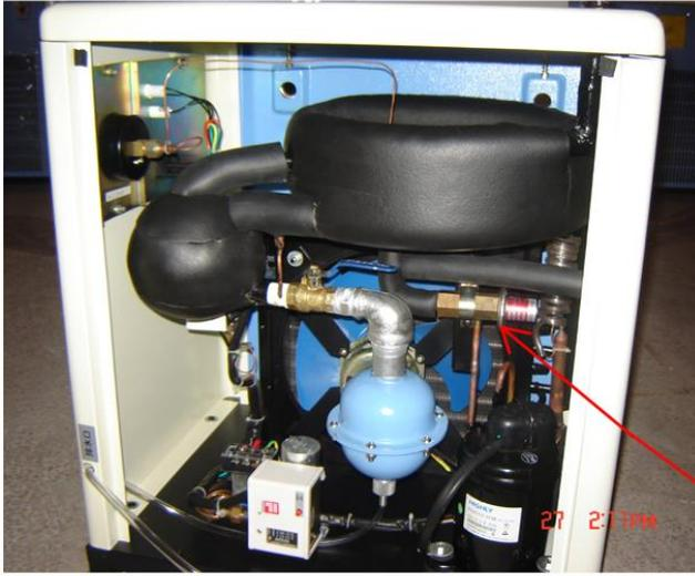
*The Hot Gas By-pass Valve need to adjusted.*
